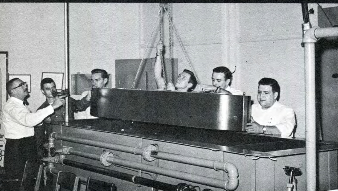
Mr. Erneman, assisted by Tom Butler, Chris Madsen, Frank Karasinski, Ed Cascardo, and Ted Hajjar, is lowering a buoyancy specimen into a water filled tank. This specimen simulates the buoyancy of a ship, and is a basic experiment in fluid mechanics.
