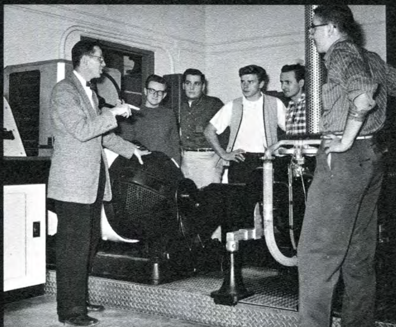
Dave Morrison, Jim Tracy, Clark Ewing, Dale Raffler, and Bob Smith look on while Mr. Chambers points out the operation of a motor-generator type of dynamometer. The dynamometer is used to check the performance of internal combustion engines.
