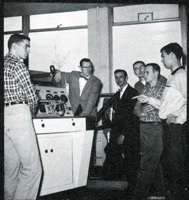
Mr. Chambers is discussing the control panel for the dynamometer with William Flower, Curtis Hay, Bob Smith, Dave Gaden, and Allen Abke. The control panel measures the fuel-air ratio and the volumetric efficiency of internal combustion engines.
