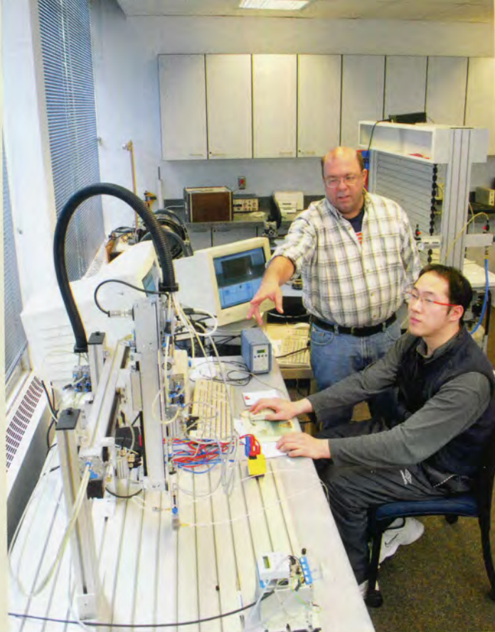
Lab Technician Mark Schmidt and automotive engineering graduate student Di Zhu collect data on a two-degree-of-freedom robot with a pneumatic drive donated by Festo Corp.
