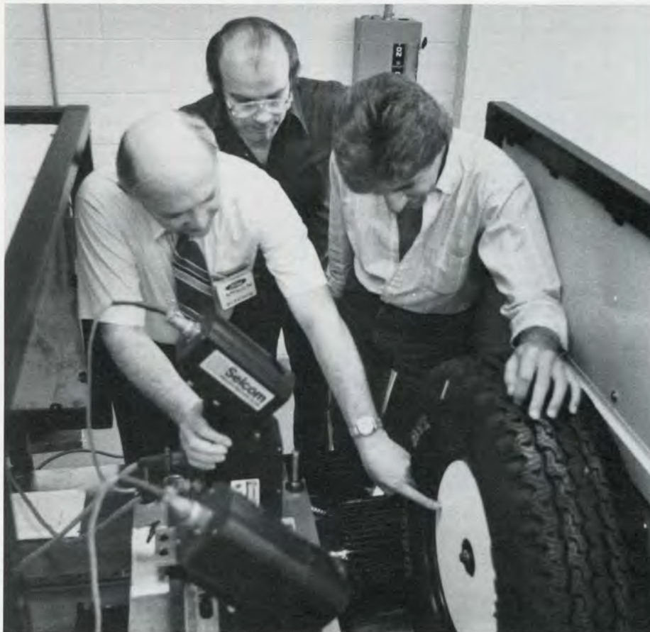
Dr. Amnon Sitchen, (left) a technical specialist with Ford's Light Truck Suspension Design and Development department, Dr. Richard Lundstrom, (center) professor of engineering, and student Marc Sarkissian inspect the spot lasers used to measure wheel alignment in a research project at LIT's new vehicle dynamics lab. The lasers were provided by Selcom, Inc., a company based in Sweden.
