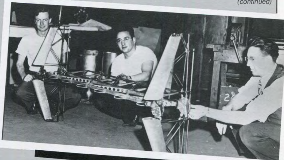
In this 1947 photograph, (L to R) Jack Walden, ArE'49, Charles Vranian, ME'49, and Prof. George Martin work on the tail section of the Spirit of Lawrence Tech. The tail was the first aircraft part assembled by the student builders.
