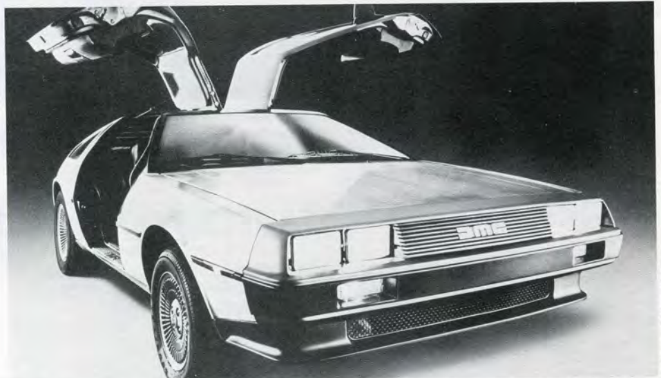
The DeLorean sports car, one of the most eagerly anticipated new automobiles in history, is now rolling off alumnus John Z. DeLorean's, IE'48, assembly lines in Northern Ireland. The car features a number of innovations, including a stainless steel skin over a glass reinforced plastic underbody.
