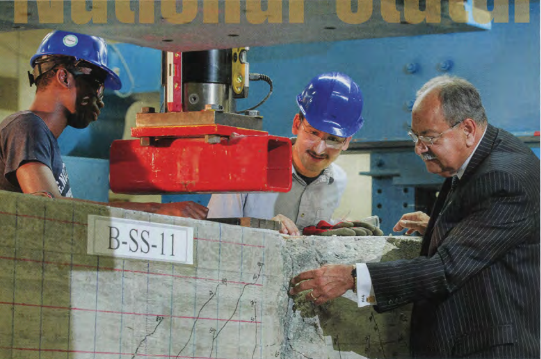
Dean of Engineering Nabil Grace (right) and his researchers have taken dozens of concrete beams to the breaking point in order to analyze the effectiveness of different materials.
