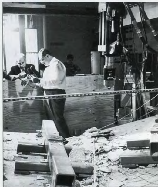
Prof. Grace (right) confers with his collaborator George Abdul-Sayed, a professor from the University of Windsor, as the two inspect a carbon fiber stirrup drawn from the debris of the third model. The 25'-long span was finally collapsed after the equivalent of 7 million heavy vehicles had passed over it, and after holding up to 135,000 lbs per sq. inch. Reinforced entirely with carbon fiber and glass fiber components, this bridge included carbon fiber stirrups which had to be custom made for the project by Mitsubishi.
