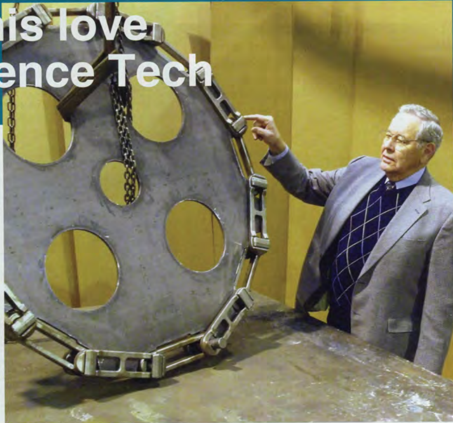
Lawrence Tech alumnus A. Leon Linton inspects a new drive sprocket that is part of an assembly capable of moving more than two and one half million pounds of live load on a single conveyor.
