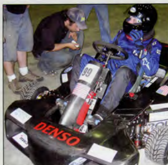
The Element One student team designed and built this racing kart powered by a hydrogen fuel cell for the Formula Zero race in Rotterdam last year.
