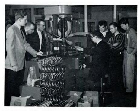
The members look on as one of the guides explains the method used to check the load limit of coil spring.
