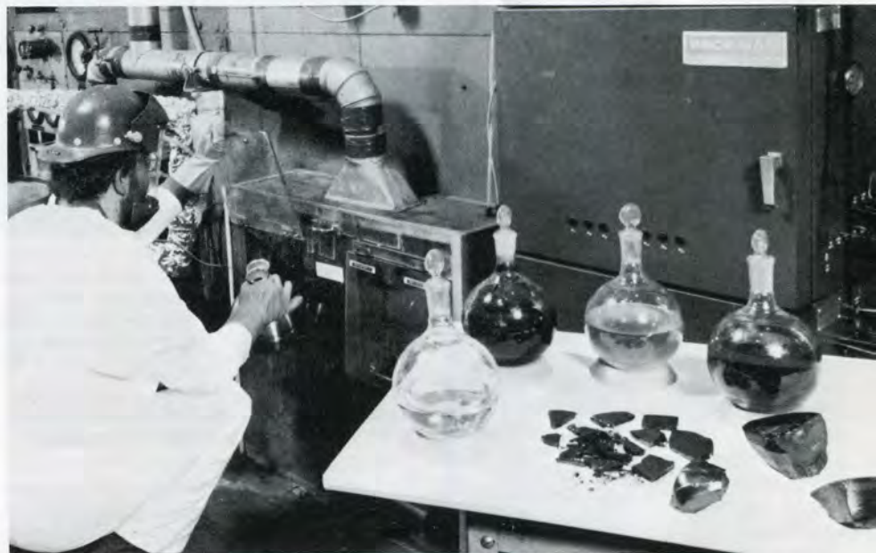
Samples of liquid fuels that can be produced from coal by solvent refining are examined by an engineer at an Air Products and Chemicals, Inc. pilot plant. The shiny black chunks are clean-burning solvent-refined coal, also manufactured by the SRC-1 process. Liquid fuels are comparable to high-grade crude oil and can be used as gasoline refinery feedstocks, boiler or turbine fuel or petrochemical feedstocks.
