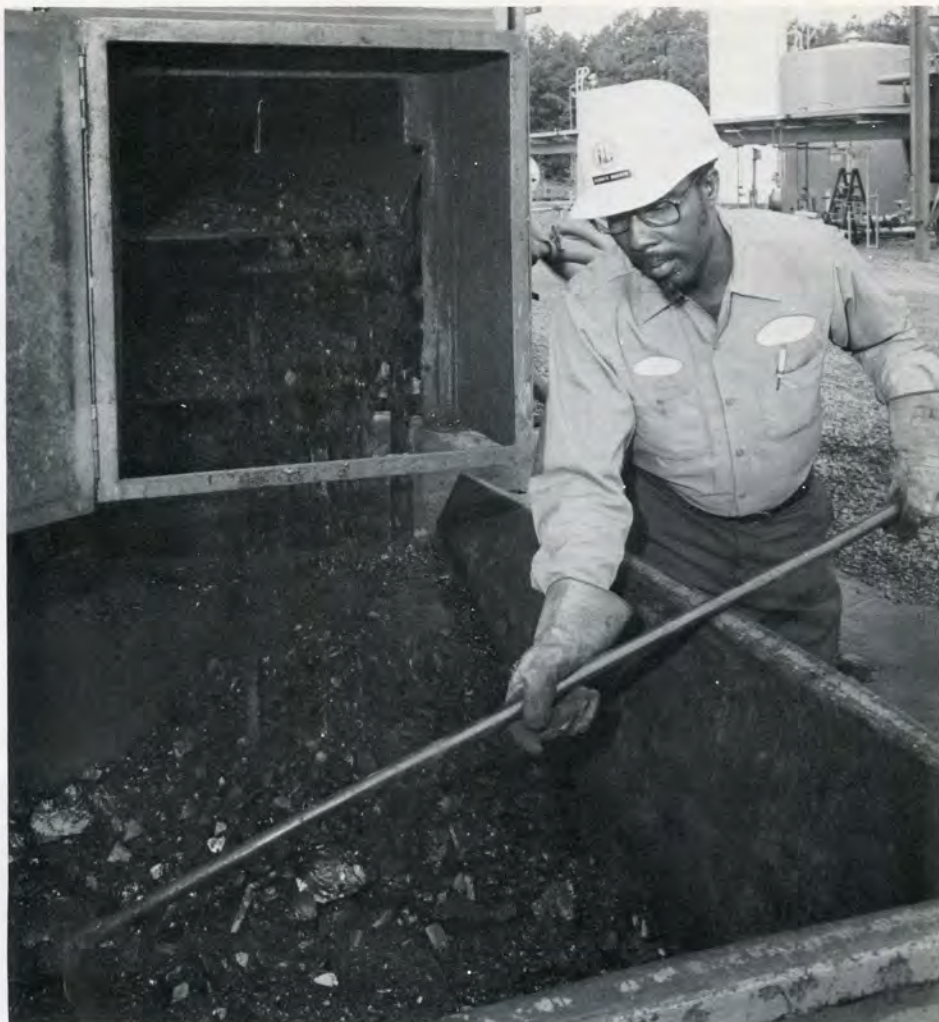
Shiny chunks of solvent-refined coal tumble off the production line at Air Product's coal refinery pilot plant operated since 1974 in Alabama. The plant turns soft coal of high sulfur and ash content into clean-burning solvent-refined fuel that can be burned as is or further processed to produce coke for the aluminum and steel industries. A second stage can be added to the SRC-1 process to convert the solvent-refined coal into a liquid fuel that can be refined into gasoline or petrochemical feedstocks.
