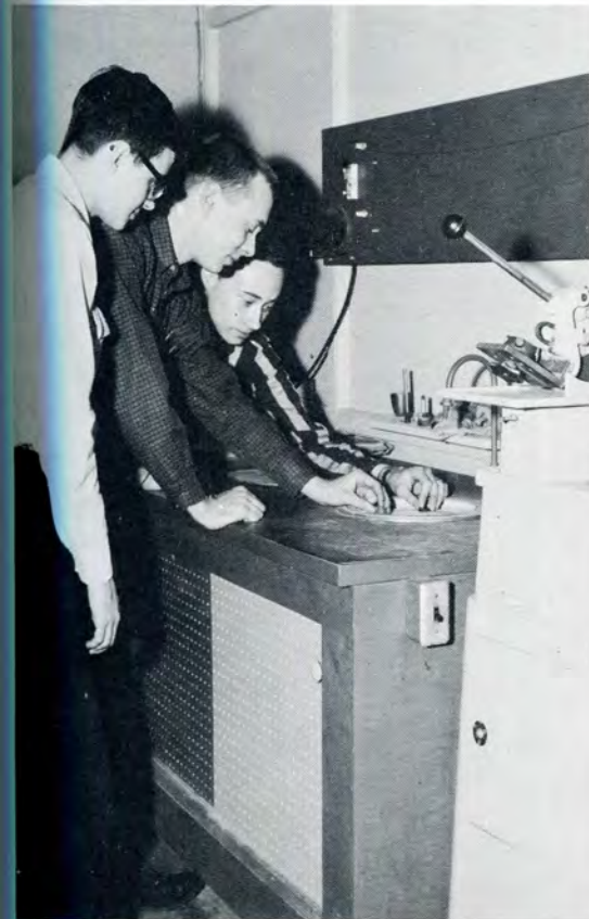
Metallurgical specimens receive watchful attention as they are polished for microscopic examination.
