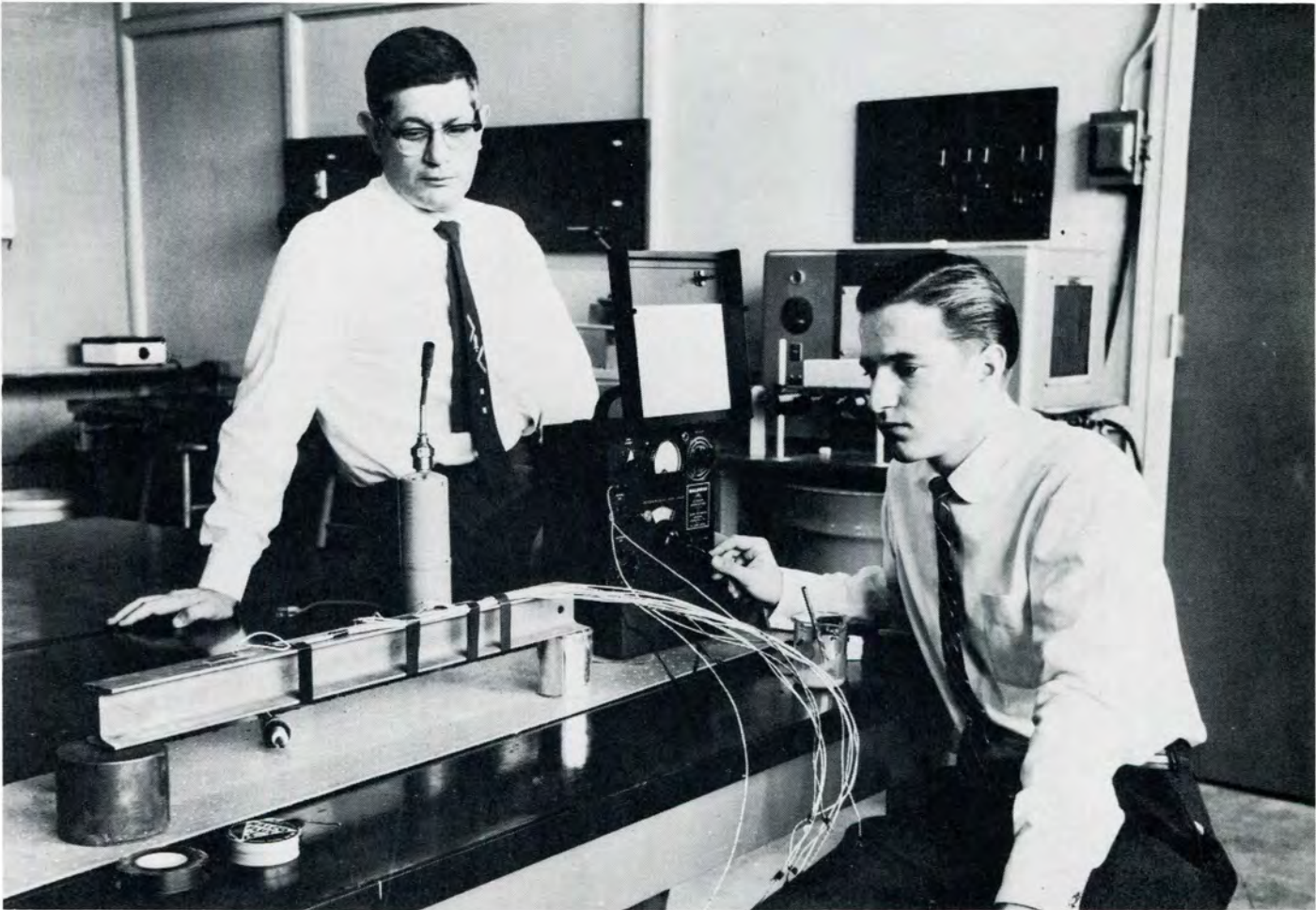
Mr. Levinson and student find the deflection of a beam through the use of strain gages.
