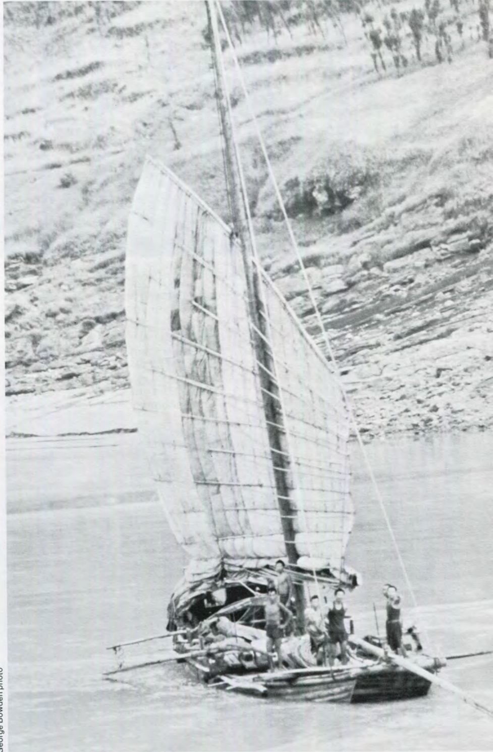
A typical vessel carrying products on the Yangtze River is a family operated "junk." They lumber up and down the river under sail, by oar, or by being towed.
