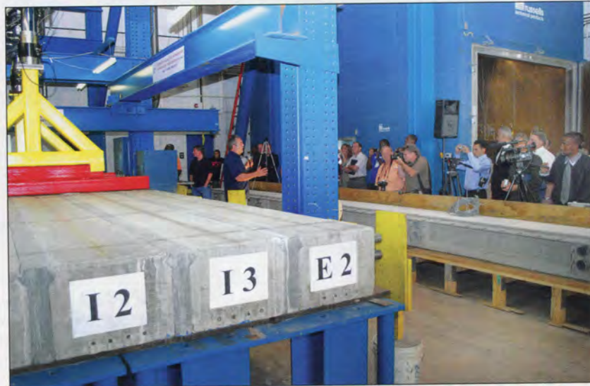
Lawrence Tech Project Engineer Charles Elder, BScME'04, describes the process for testing a pre-stressed decked bulb-T beam bridge (in the foreground) to an audience that included government officials and media representatives.
