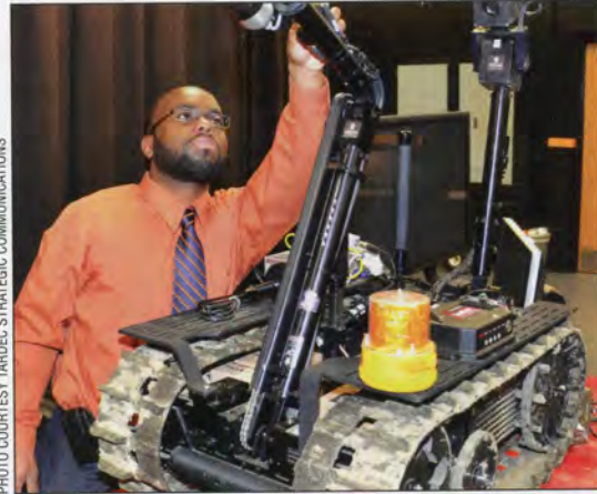
Christopher Scott examines a ground robotic vehicle that has been designed to locate and neutralize explosive devices in combat zones.
