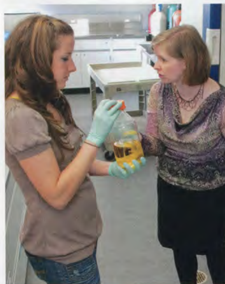
Molecular and cell biology senior Samantha Hartner and Assistant Professor Julie Zwiesler-Vollick check to insure that the bacterial growth medium is thoroughly dissolved and the cap on the bottle is loosened prior to steam sterilization in the autoclave.
