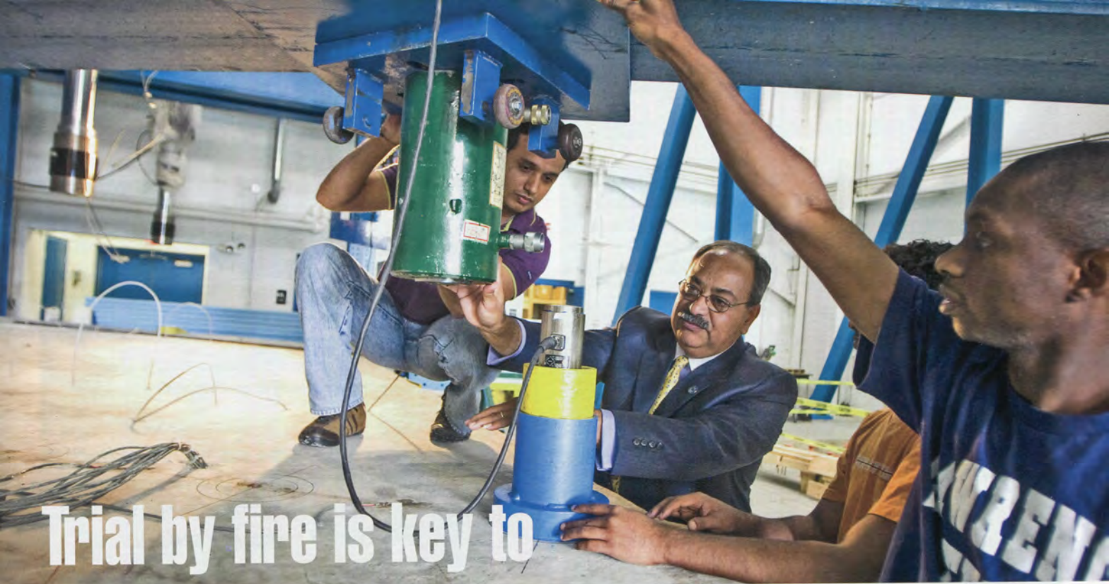
Nabil Grace and students working at the Center for Innovative Materials Research (CIMR) prepare a hydraulic actuator for a load distribution test.
