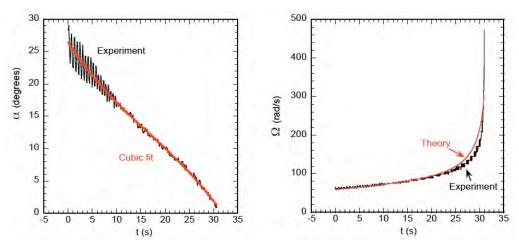
The above data was collected from time-lapse photographic measurements of the spin of a PiTOP prototype that I sent for analysis to Professor Rod Cross at the University of Sydney, (cf. "Effects of Rolling Friction on a Spinning Coin or Disk", *European Journal of Physics*, 39, #3, 5, 2018).
