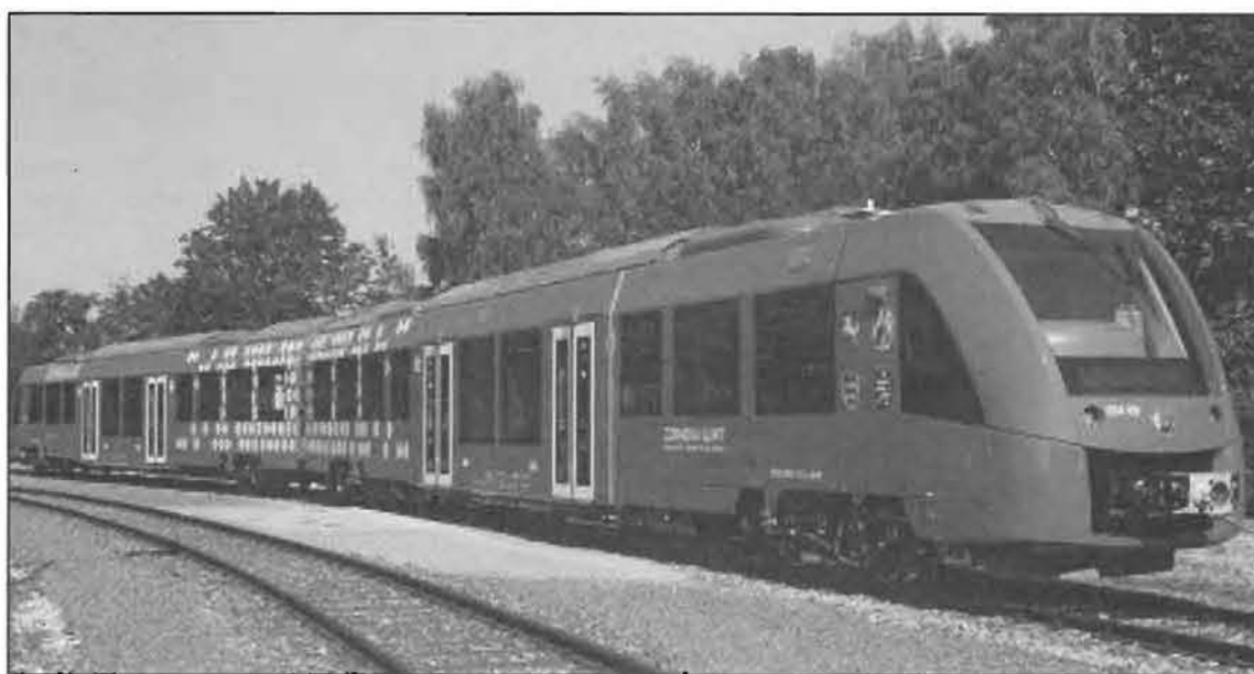
Coradia iLint, Germany's new hydrogen train, is set to go into service in December 2017.
