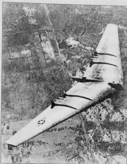
THE WAVE OF THE FUTURE - YB-49 Flying Wing. Wing span - 172 feet.
