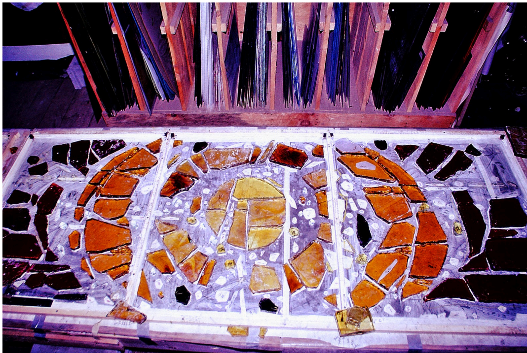
The center window of three dalle de verre windows for St. Joseph Catholic Church, Wakefield, Massachusetts . The uncut glass sheets at the top are for leaded glass work, not the dalle de verre that Robert was working on. Some of the cut glass pieces for Robert's work--but not all--are laid out on the full-size cartoon. The three chapel windows, fabricated by the Cummings Stained Glass Studios in 1980, are below. (Above photo courtesy of Robert Pinart; photo below courtesy of Merry Nordeen and St. Joseph Church)
