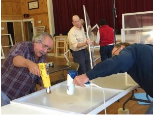
Belfast/Searsport Window Dressers is a volunteer organization that helps local residents by reducing heat loss through their windows.
