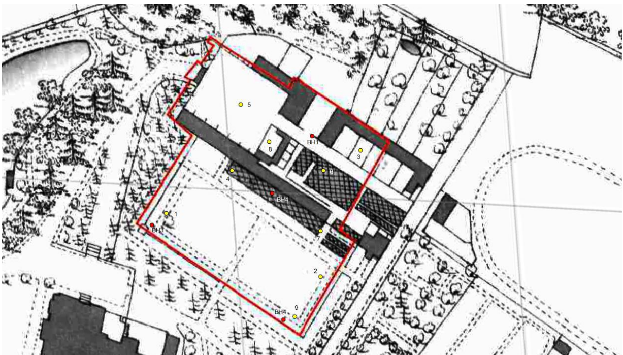
Figure 2. Locations of boreholes and watching brief geotechnical pits (Wellicome, 2013).
