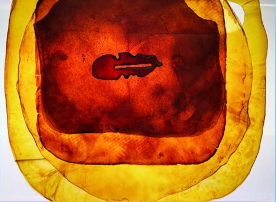
Samples of vegan leather made from dehydrated SCOBY (Symbiotic Culture of Bacteria and Yeast). Courtesy Saad Chinoy / Edible Makerspace.
