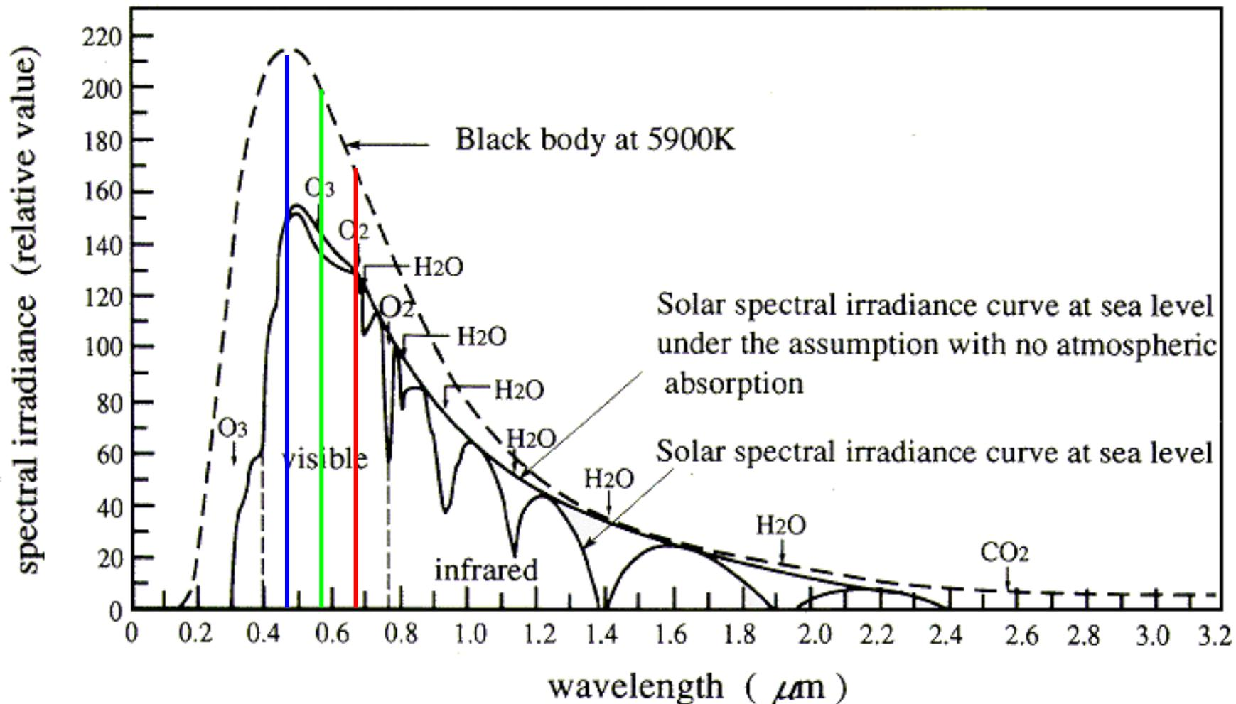
**Comparison of spectral irradiance of solar light at sea level with black body radiation**
