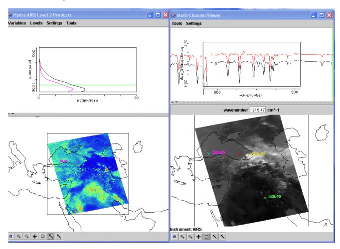
**Figure 4.** (right) MultiChannel Viewer display with zoom in on IR window spectra near 870 cm-1 over FOVs in eastern and western Black Sea. (left) AIRS water vapor profile retrievals in the two selected FOVs and the 900 hPa water vapor retrieval field for the granule.
