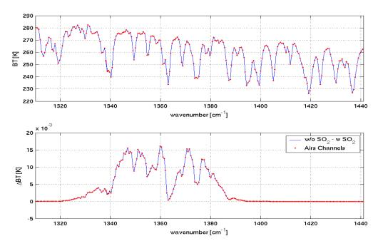
The top panel of this figure shows one simulated AIRS spectrum in the region that goes from 1320  $cm^{-1}$  to 1441  $cm^{-1}$ . The bottom panel shows the differences between the simulated AIRS spectrum with and without SO<sub>2</sub>.
