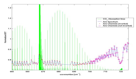
5. This plot shows an AIRS normalized spectrum (blue) along with the CO2 lines (green). In the spectral regions where the red dots indicate the AIRS channel the online channels are warmer than the offline channels, can you explain why? In the spectral region where the magenta circles indicate the AIRS channels the on-line channels are colder than the off-line channels, what is the difference between the two spectral regions.
