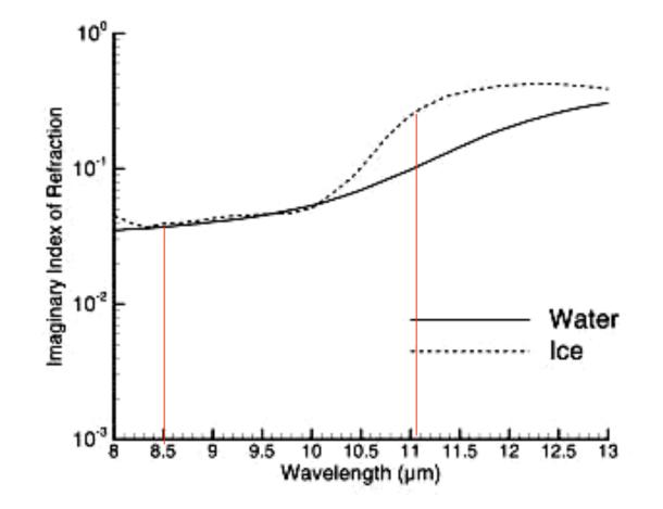
Imaginary Index of Refraction of Ice and Water 8-13 microns
