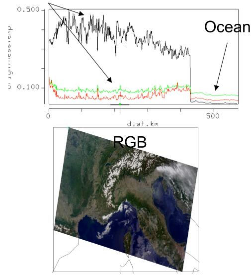
NIR (.86 micron) Green (.55 micron) Red (0.68 micron)
