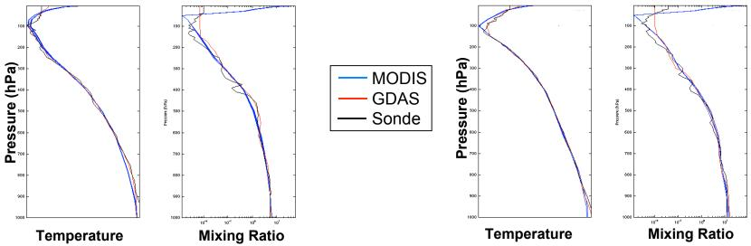
But not so well with smaller-scale features, such as isolated dry or moist layers:
