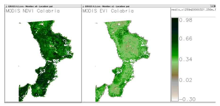
Both NDVI and EVI maps are colored with identical color table (MODIS/Terra scene MOD13, composite of 21 March - 5 April 2000, Calabria, Southern Italy). EVI is less prone to atmospheric distortion (from http://mpa.itc.it/rs/modis\_ndvi\_evi/)
