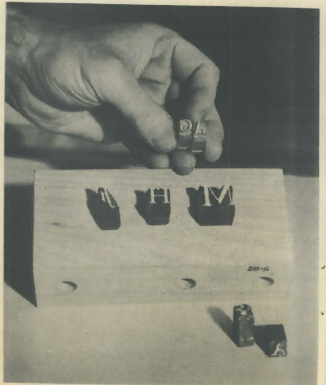
Original type punches, hand-cut by William Caslon, recently presented to CW by Harry Porte of New York.
