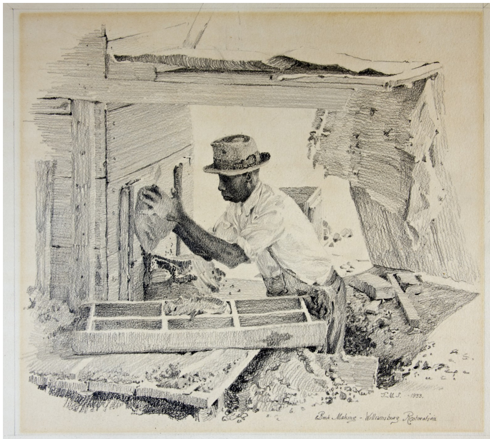
Bob Sowers filling brick molds at the pug mill of the Todd and Brown Inc. brickyard, 1933.
