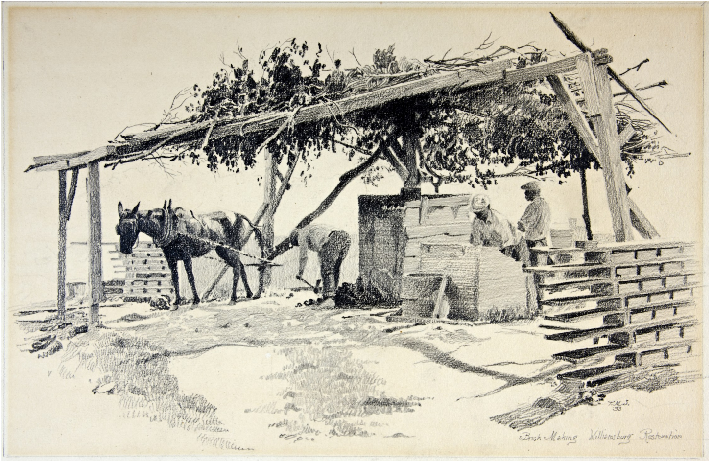
Colonial Brickyard Company workmen operating the pug mill at the Todd and Brown Inc. brickyard, 1933.
