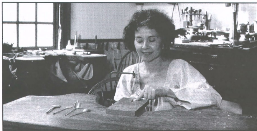
Journeyman silversmith Gayle Whiting uses a jeweler's saw to craft the decorative details of a tea strainer spoon.
