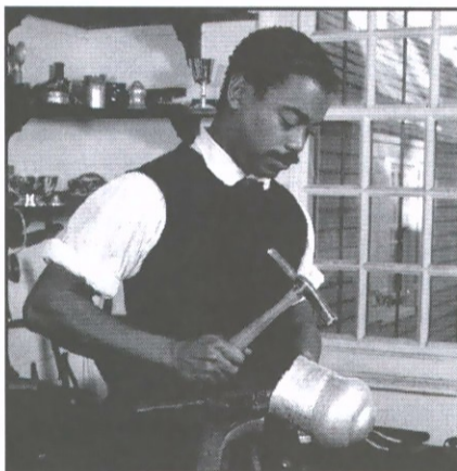
Silversmith Preston Jones Jr. hammers silver into what will soon become a tea kettle. Photo by Tom Green
