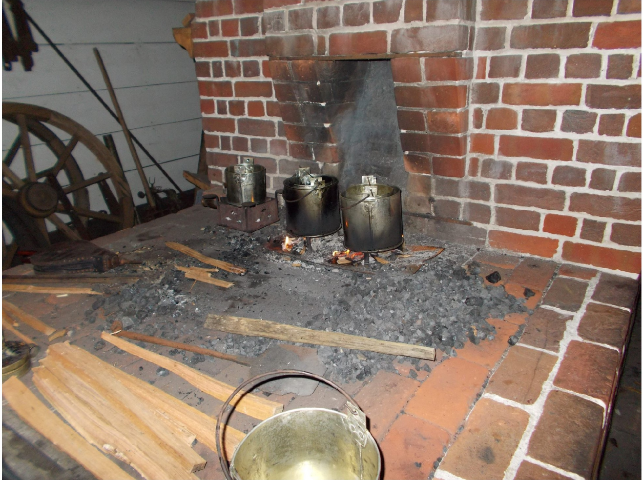
Three sets of double boilers, one of tallow, one of beeswax and one a combination of both.
