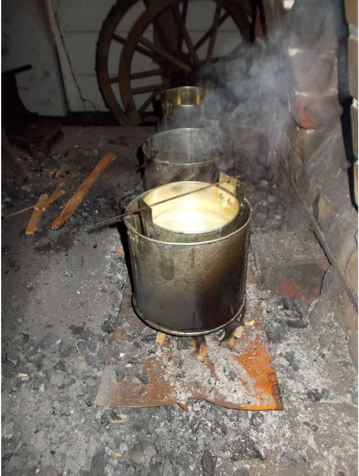
Three sets of double boilers, one of tallow, one of beeswax and one a combination of both.
