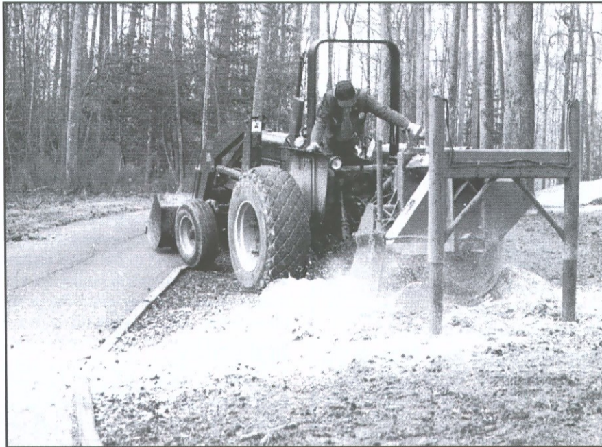
Cutting dead trees down is just half the job. A large power saw mounted on a tractor grinds away the remains of the stump left in the ground. Trees that are removed from the course are replaced with new trees.
