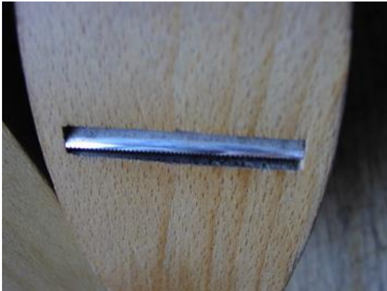
Toothing plane blade edge (left) and toothing plane surface on veneers (right).
