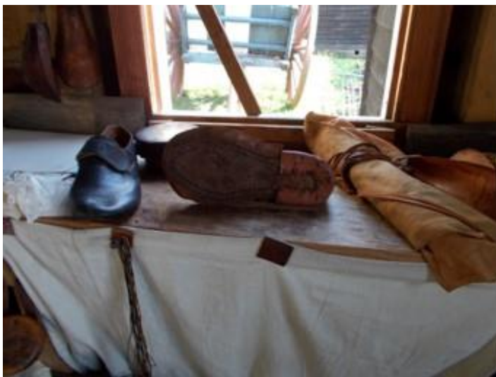
The welt and rand have been sewn into place for the second of a pair of common shoes for David Wilson.
