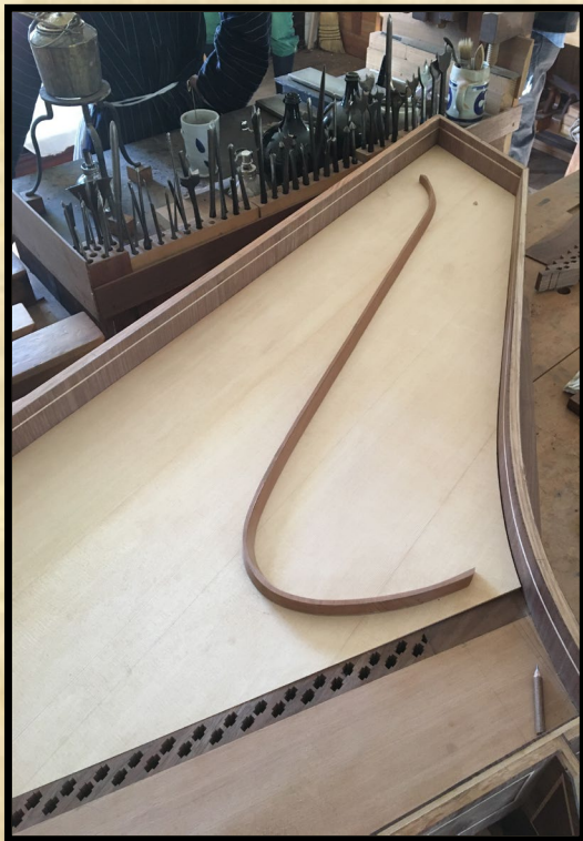
The cherry bridge strip in position in the spinet.
