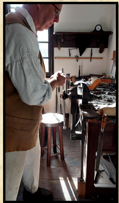
Brad drilling through the lock plate with the brace & bit.
