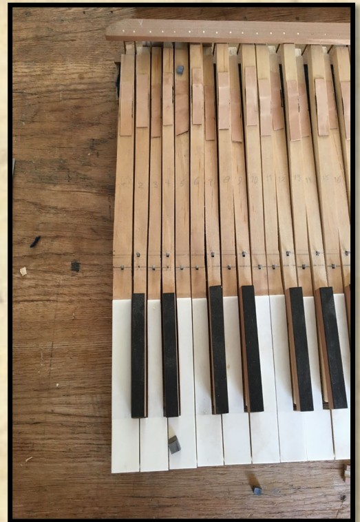
Keyboard with balancing lead weights.
