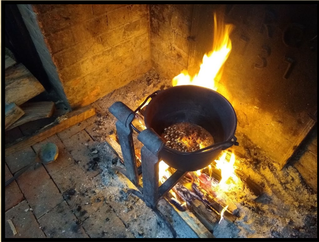
Cast musket balls are remelted as raw material for a new cast batch.
