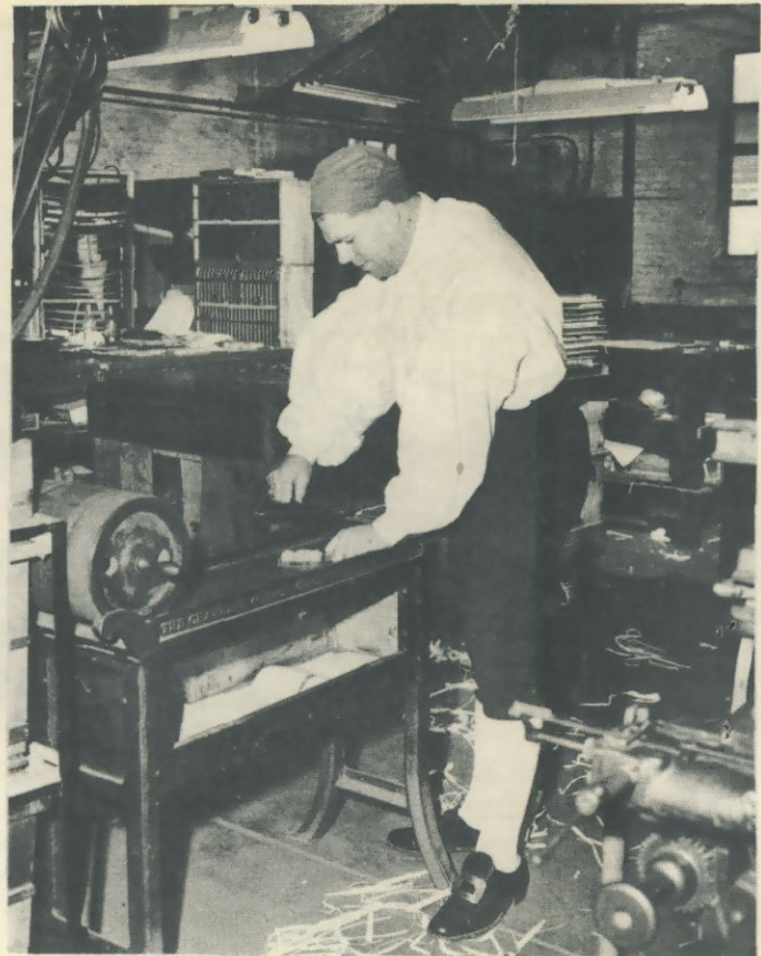
August Klapper borrows the modern Virginia Gazette plant to pull a proof from 18th century type for the Printing Office.
