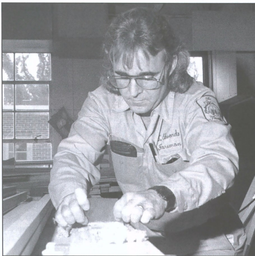
Tim Edwards in the millwork shop scrapes one of the mantelpieces that are to be installed at the George Wythe House.
