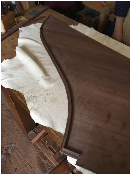
Lid curve refined to match the molding and case
