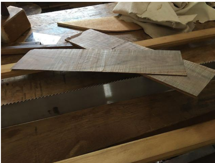
Veneer sawn at 1/32 inch with the veneer saw
