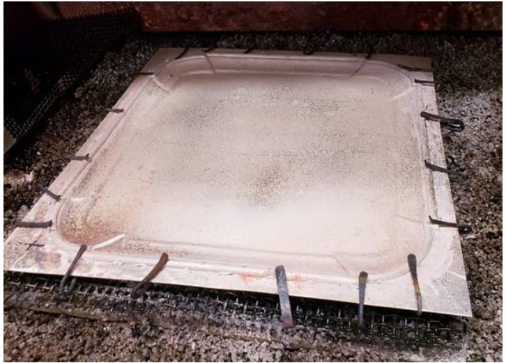
Bobbie's tray: The iron clips are holding the silver rim in place so that it can be soldered together.
