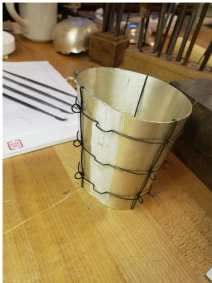
A seamed cup bound in iron wire and being prepped for soldering
