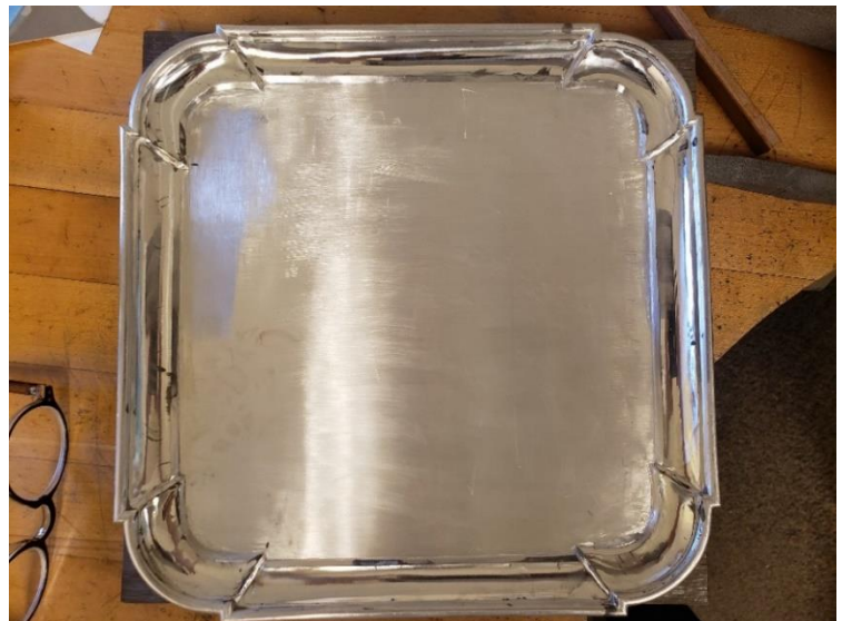
A seamed cup bound in iron wire and being prepped for soldering
