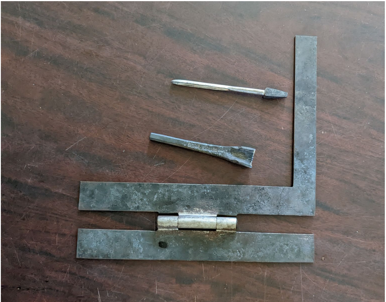
An H-L hinge, a pinking iron, and a spoon bit for a brace.
