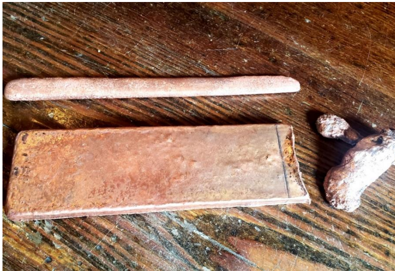
The copper ingots along with a nugget of overspill
