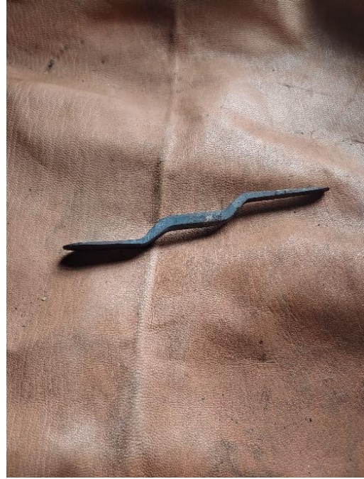
One of the Small Tools made for the Brickmakers. Notice the bends and flat pointed ends.
