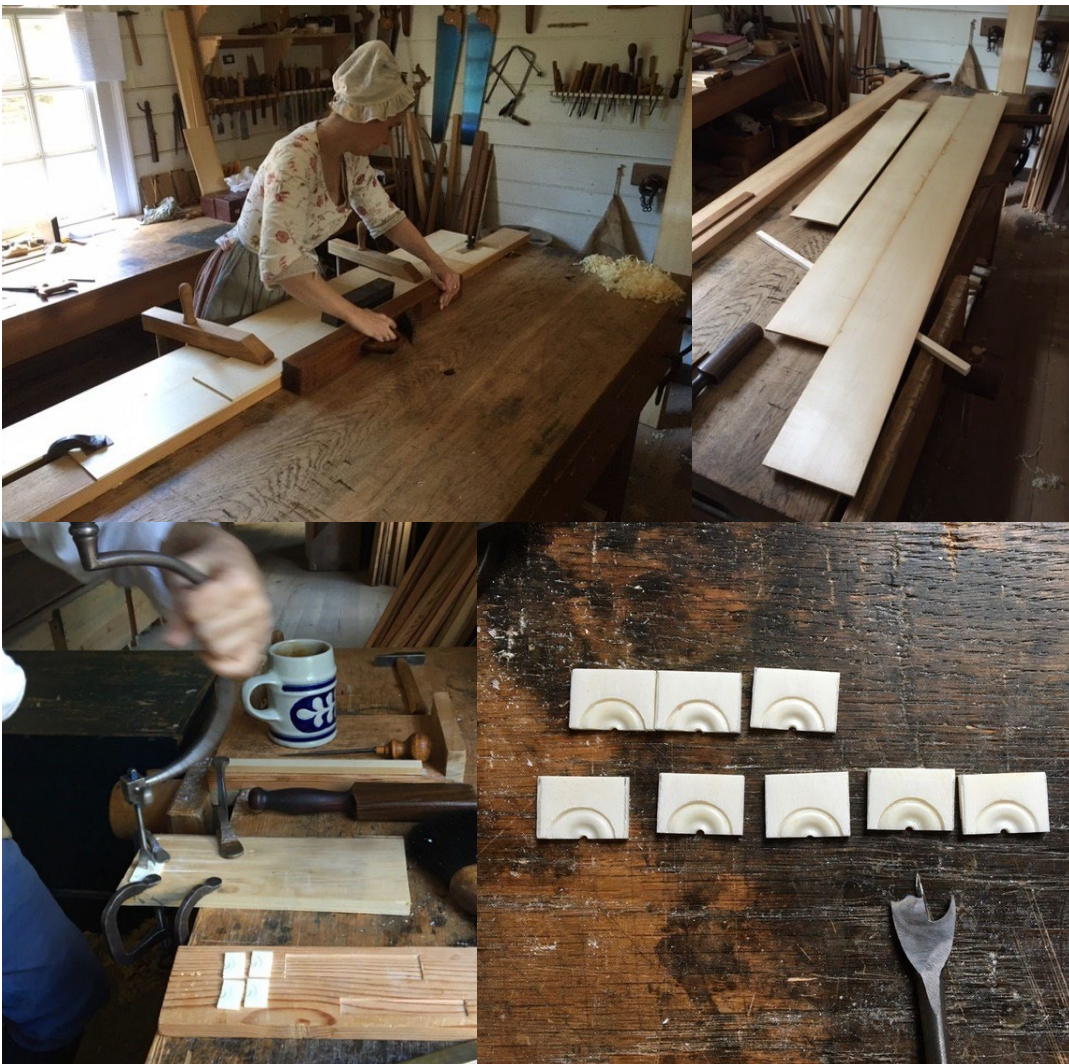
Clockwise from top left: Melanie Jointing Soundboard Pieces by Planing. Soundboard Pieces Beigh Glued. Ed Drill Arcade Profiles Finished Arcades for Natural Keys
