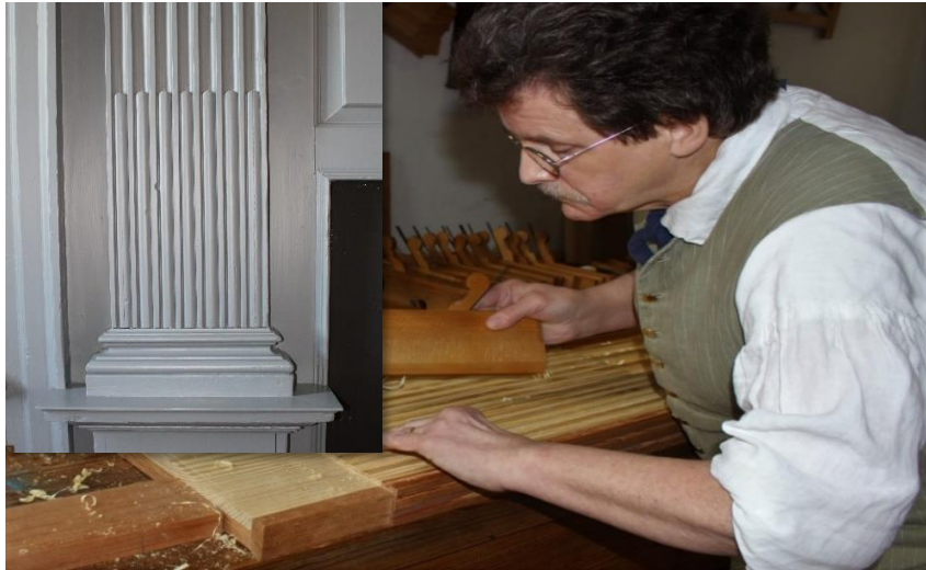
Brian is refining the reeding on the Warren House Pilaster using a hollow moulding plane.
