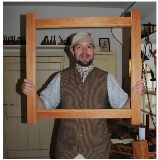
Scott assembling the mortise and tenoned frame for the lower door of the cupboard
