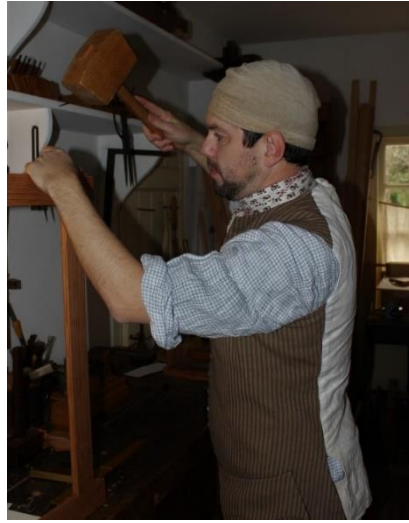
Scott assembling the mortise and tenoned frame for the lower door of the cupboard
