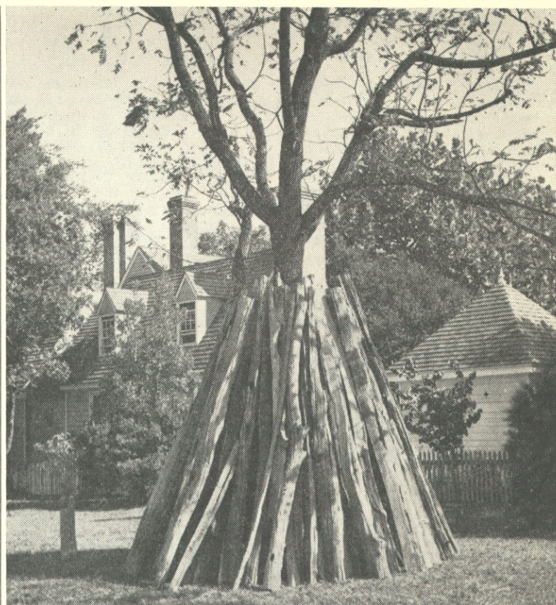
LUMBERING ALONG — In the 18th-century, colonial householders used trees as drying racks for split chestnut and oak logs which they planned to use in the construction of the rail fences that are so familiar in Virginia. The system was effective, since it allowed the air to get to the logs with a minimum of exposure to the dampness of the ground. It also took considerably less space than it would if they were to be piled up on the ground. Partially for atmosphere and partially for drying purposes, CW has piled up split logs at the trunks of five trees in the restored area. The logs will be used later to construct a rail fence that will surround the site of Robertson's Windmill. Photo by George Beamish
