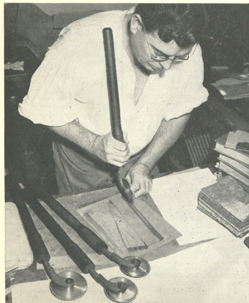
ROLLAWAY — Bookbinder Clem Samford demonstrates one of the four reproduced rolls which will be used in his work. The rolls impress a design on the leather. To impress the design in gold, a roll is then heated, touched to the gold leaf and then run over a previously-impressed design, leaving gold leaf in the design. Photo by George Beamish
