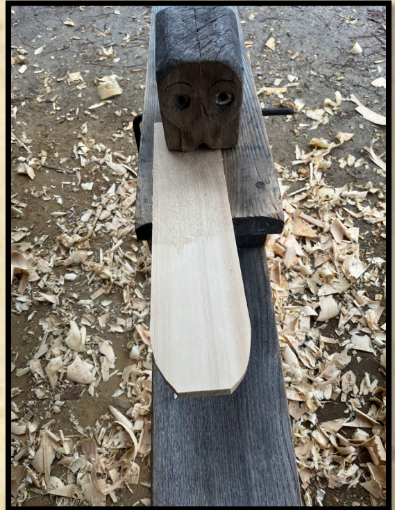
A finished shingle ready to go.
