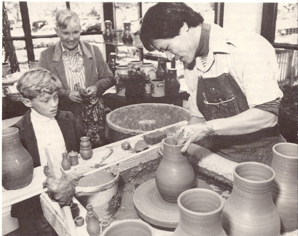
David Chong from the Williamsburg Pottery showed customers how he compensates for shrinkage during firing by throwing bird bottles that are 10 percent larger than the final reproductions.
