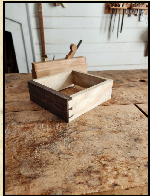
Tamsyn's first drawer, with half-blind and through dovetails
