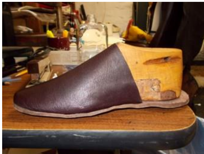
The slipper has been turned right side out and is drying on the last. Since the sole is curved, and we want the top piece of the heel to be level, the split-lift acts as a wedge, allowing that to happen.
