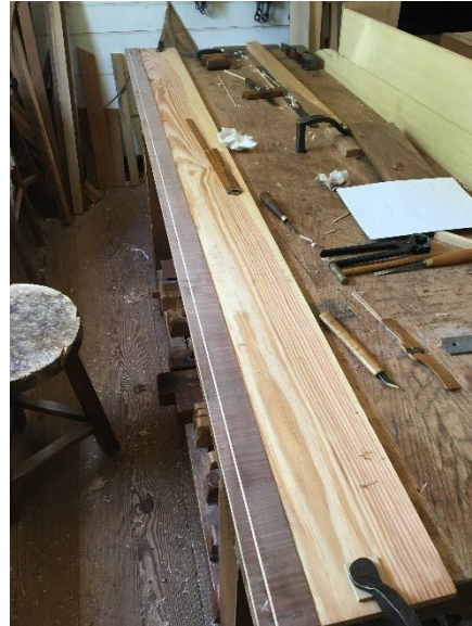
Backboard inner veneer after gluing (left). Backboard inner veneer with strip inlaid and smoothed (right).
