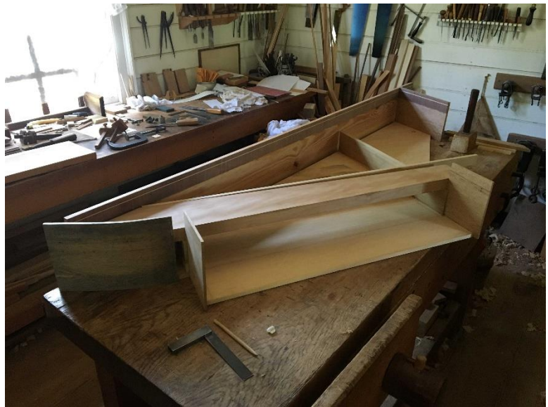
Fitting the keyboard flank cheek walls into inner assembly (left). Spinet parts laid out in situ pre assembly
