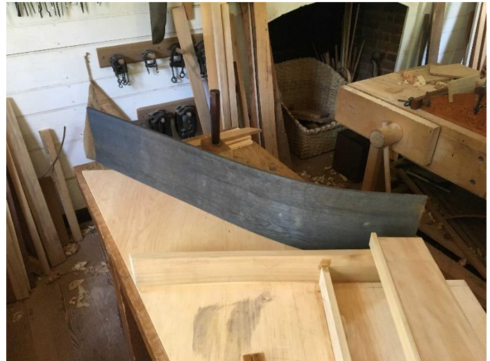
First bentside with unfortunate damage in situ
