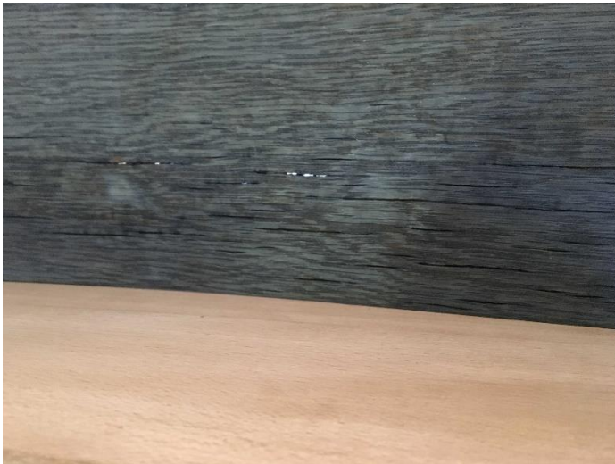
Cracks in bentside showing through light
