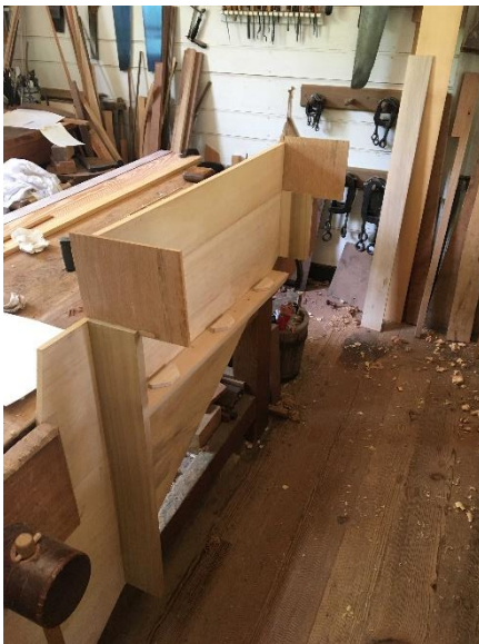
Fitting the keyboard flank cheek walls into inner assembly (left). Spinet parts laid out in situ pre assembly
