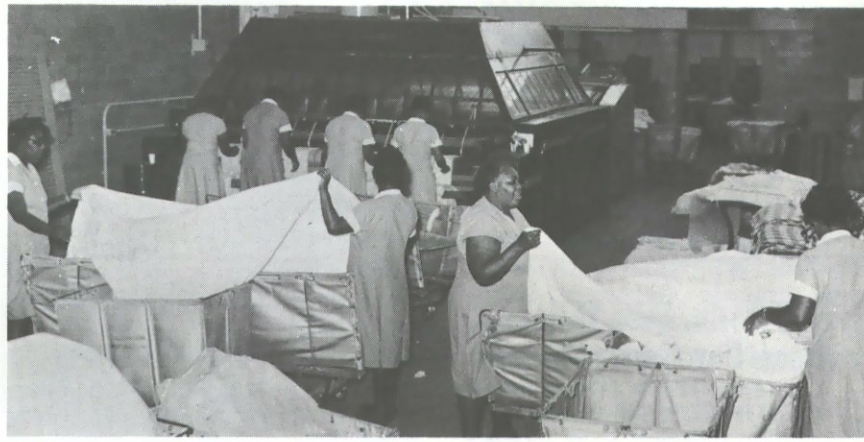
CWers are shown here preparing sheets for the flatwork ironer, shown top left. All flatwork items are pressed and folded by this machine, which is capable of processing 1,000 sheets an hour.
